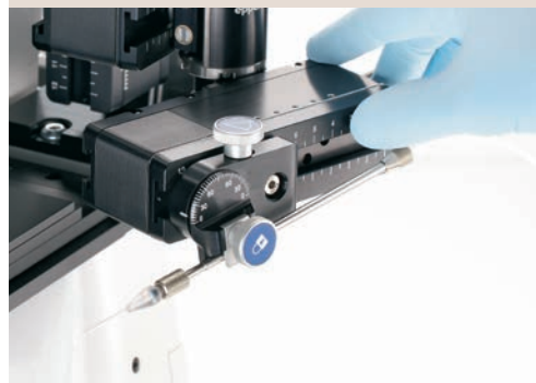
Swivel out function for easy capillary exchange.
