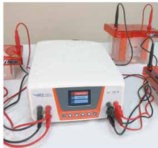
Four pairs of outlet terminals
